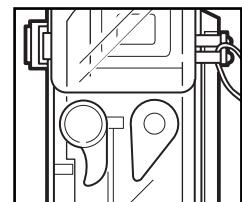
Place the included anti-fogging silica gel in the gap between the camcorder and the marine case to prevent fogging in the marine case.
