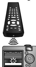
Point a digital camera towards the remote control. Push any button on the remote control and look through the digital camera. If the infrared light appears through the camera, the remote control is working.
