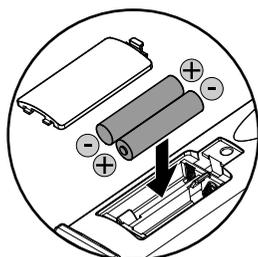
Make sure to match + and - on the batteries to the marks indicated in the battery compartment.
