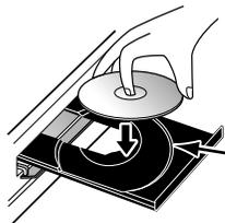
Align the disc to the disc tray guide.
