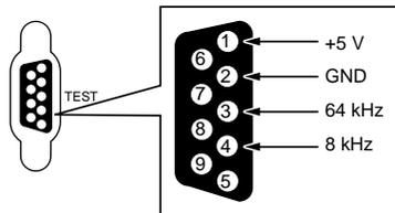
**Figure 3. DB-9 Connector Pinout**
