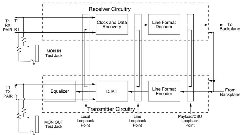
**Figure 2. Bantam Jack Monitoring Points**
