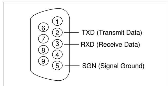
**Figure 5. RS-232 (DB-9) Pin Assignments**
