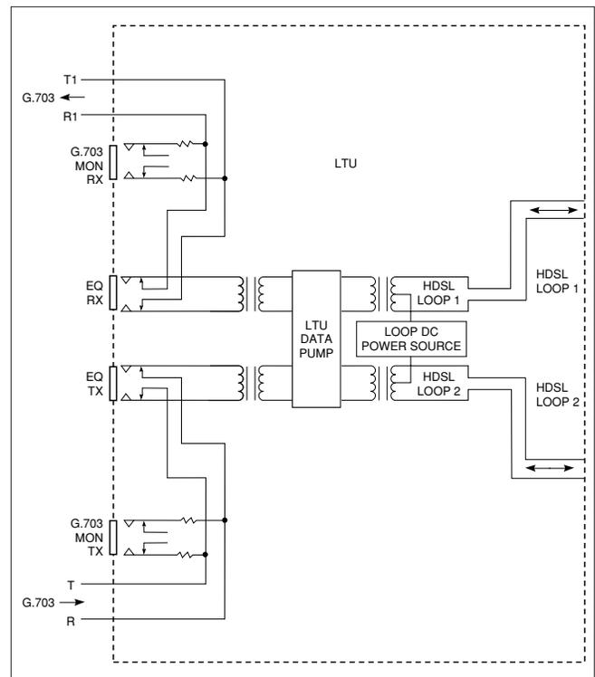
**Figure 3. LTU Span Powering Diagram**
