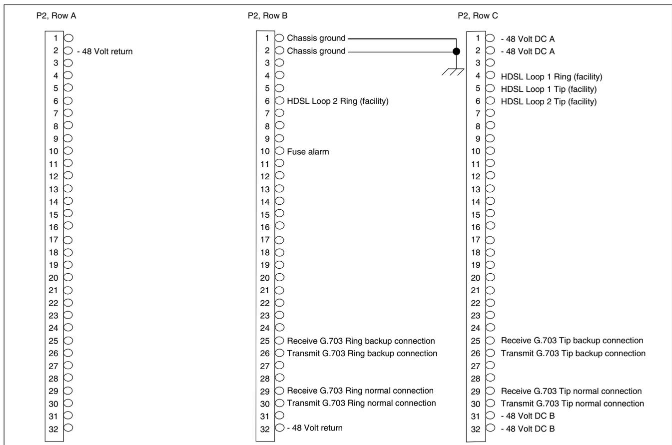
**Figure 2. LTU Edge Connector Wiring**
