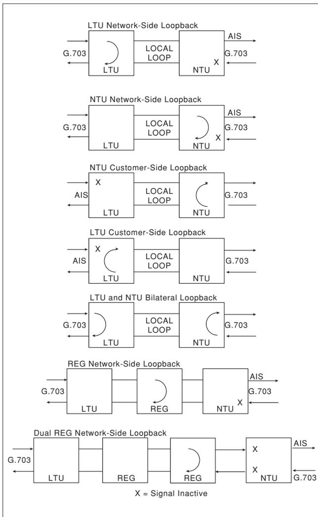
**Figure 4. HDSL Loopbacks**
