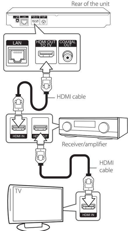
Connect the amplifier's HDMI output jack to HDMI input jack on your TV using a HDMI cable if your amplifier has HDMI output jack.
