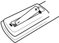
Remove the battery cover on the rear of the Remote Control, and insert the R03 (size AAA) battery with  $\oplus$  and  $\ominus$  matched correctly.
