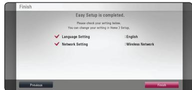
Press **ENTER** (⊙) while [Finish] is highlighted to finish the initial setup settings. If there is any settings to be changed, use **◀/▶** to select [Previous] and press **ENTER** (⊙).
