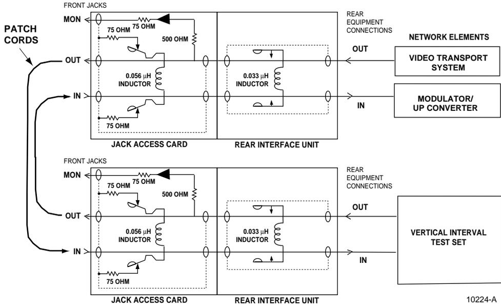
Figure 29. Insertion of Test Signal
