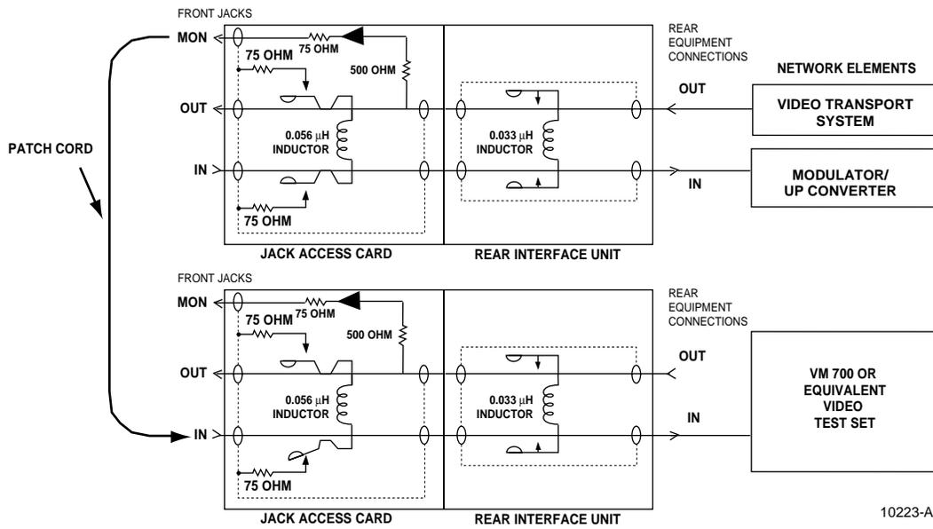
Figure 28. Non-Intrusive Test of Transport Feed
