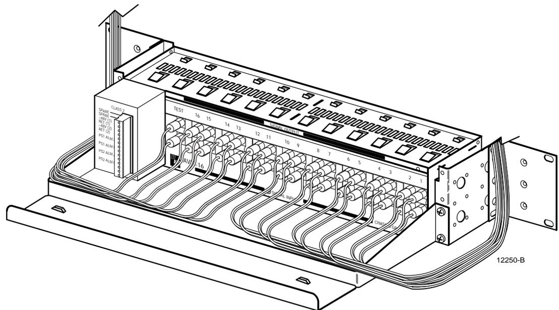
Figure 15. AVIS Chassis Cable Routing
