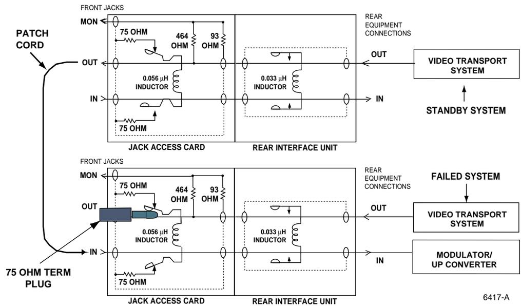
Figure 21. Bypass Failed Video Transport System
