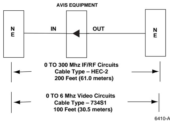
Figure 11. Recommended Maximum Cable Lengths
