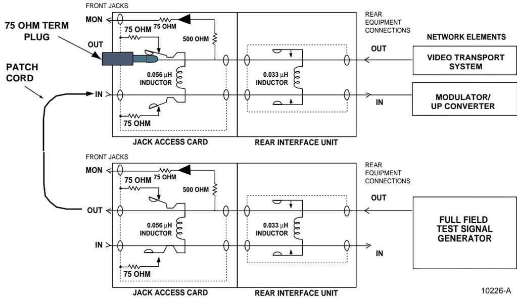
Figure 31. Intrusive Insertion of Test Signal
