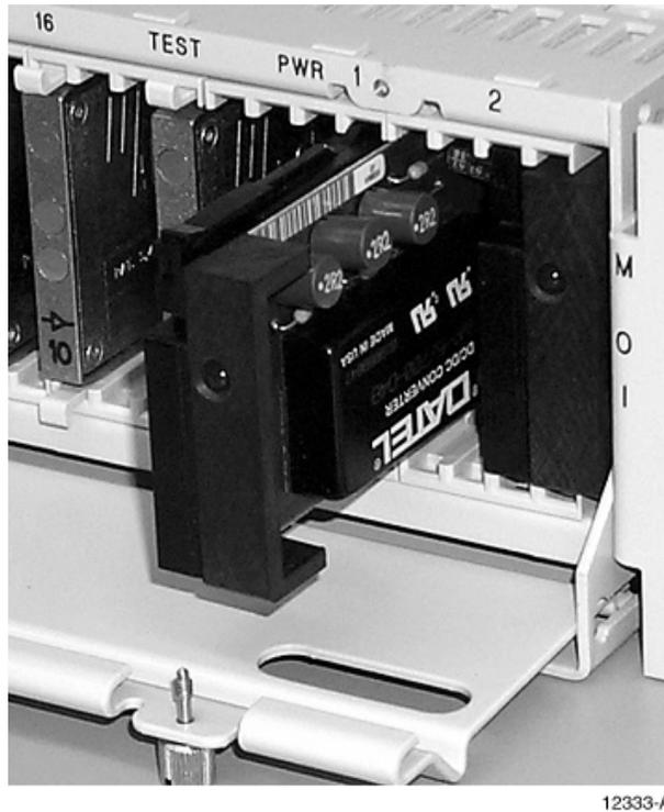
Figure 4. Power Supply Module
