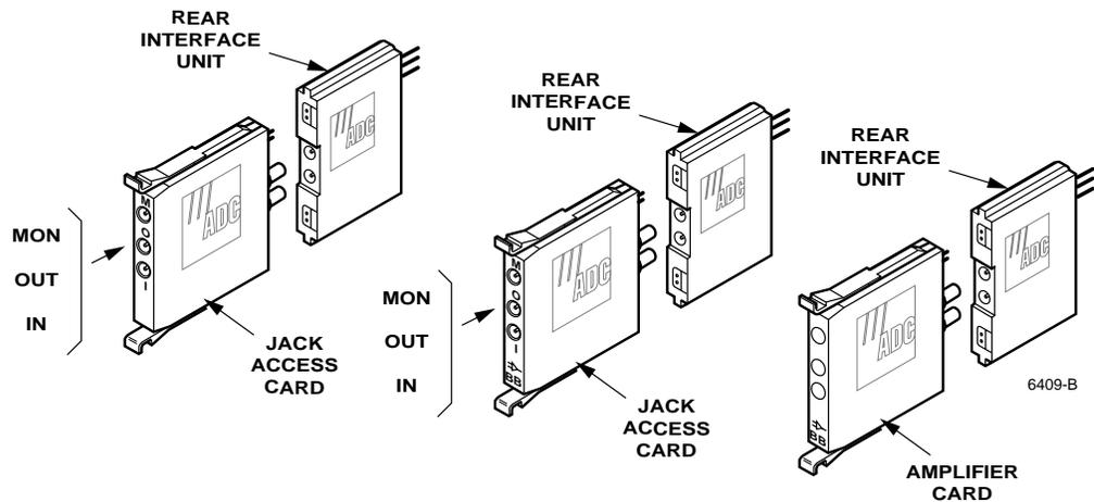
Figure 10. Passive and Active Jack Access Cards
