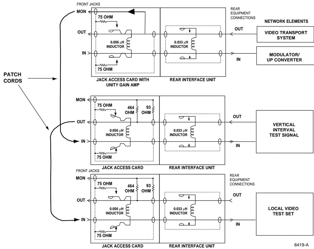
Figure 27. Non-Intrusive Insertion of Video Test Signal with Unity Gain Jack Access Card
