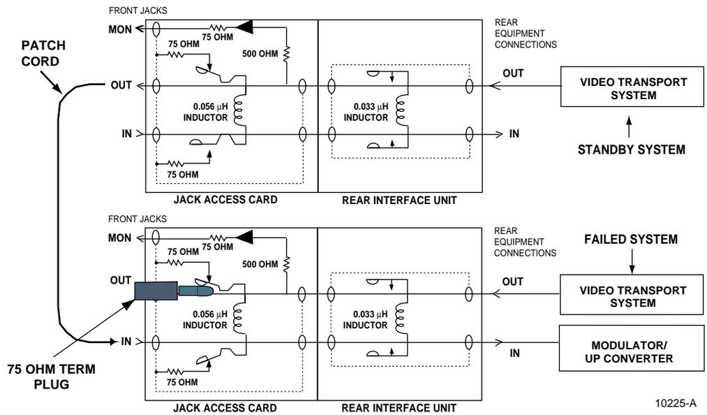
Figure 30. Bypass Failed Video System
