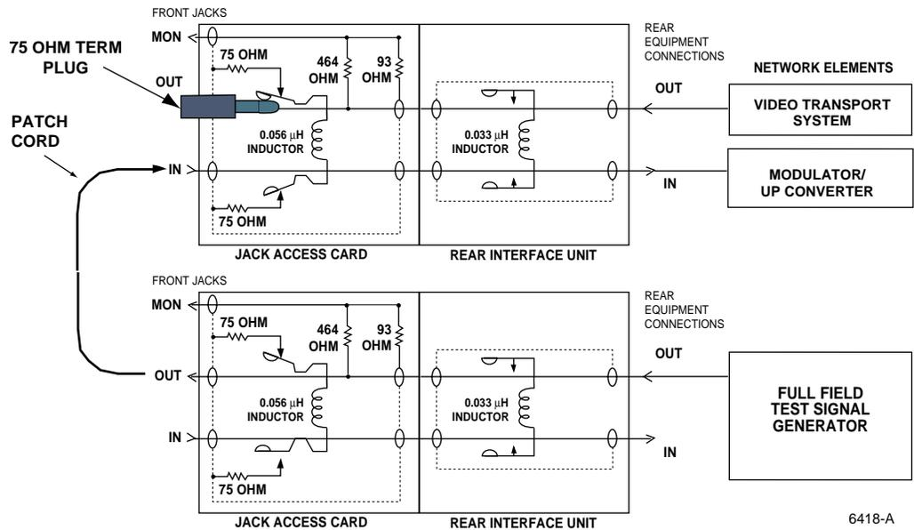
Figure 22. Intrusive Insertion of Test Signal
