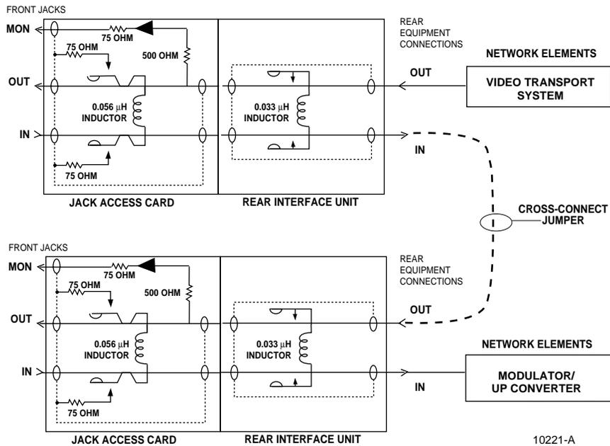
Figure 25. Typical Cross-Connect Application
