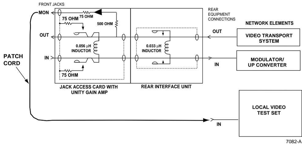
Figure 23. Non-Intrusive Video Test Access
