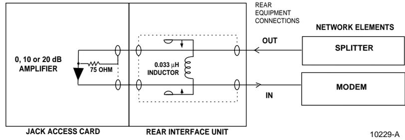
Figure 34. Typical Interconnect with Gain Application
