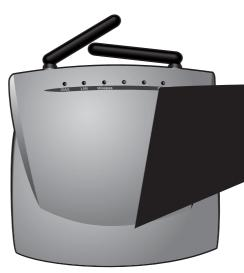
The top of your Wireless AP has four clearly labeled status indicator lights (or *LEDs*). Once your Wireless AP is installed, these LEDs display the status of the network and the condition of your Wireless AP, as described:
