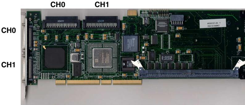
Figure 2-1. AcceleRAID 352 Controller with Connectors
