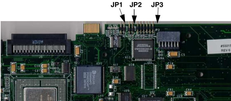
Figure 2-2. AcceleRAID 352 Default Jumper Identification
