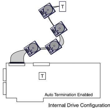
**Figure 2-10. Termination with Internal Drive Configuration**
