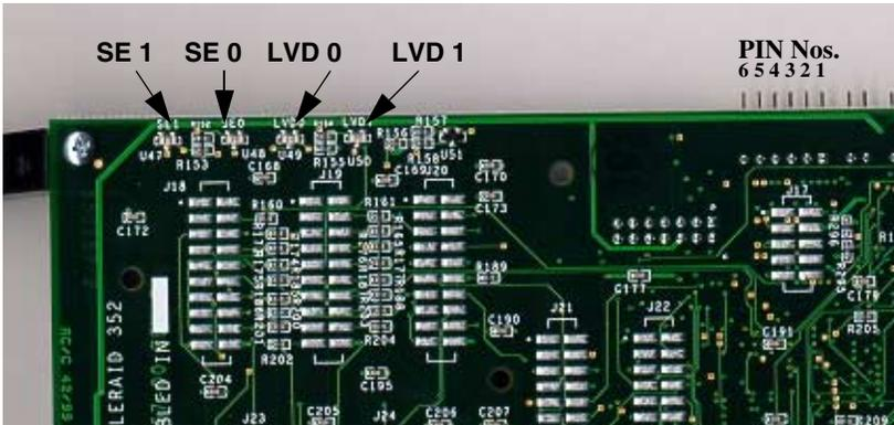
Figure 2-4. AcceleRAID 352 Controller with LEDs and Pin Numbers (back)
