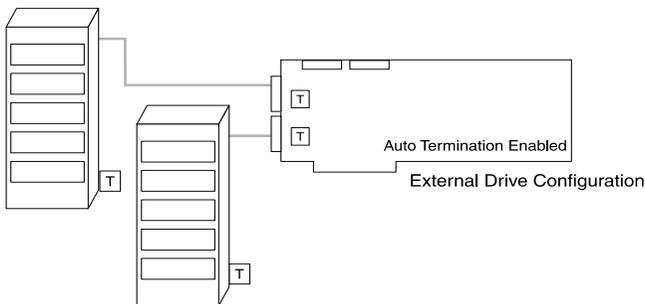
**Figure 2-11. Termination with External Drive Configuration**
