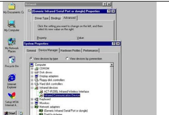
4. Highlight (**Generic Infrared Serial Port or dongle**), click **Remove** button. Then Click **OK** button.
