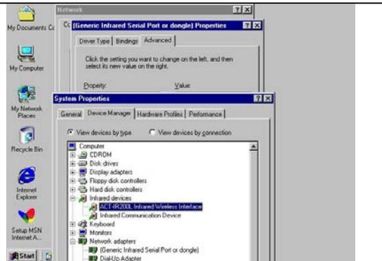
3. Highlight the **Infrared Communication Device** in the **Infrared devices**, then click **Remove** button.
