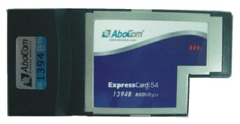
ExpressCard slot. The **E94B** also provide 1394B/FireWire functionality to your legacy Windows, Linux or Mac machine with a simple 1394/FireWire adapter Expresscard you plug into an available Expresscard slot.
