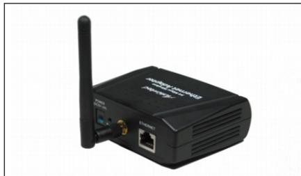
2. Get the **yellow Ethernet cable** from the package. Plug one end of the cable in **Ethernet port** on the back of the Adapter. When seated properly, the cable will “click” in the port.
