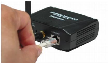
3. Plug the other end of the **yellow Ethernet cable** into the **Ethernet port** on the back of the game console (Xbox, PlayStation 2, etc.) or computer. When seated properly, the cable will “click” in the port.
