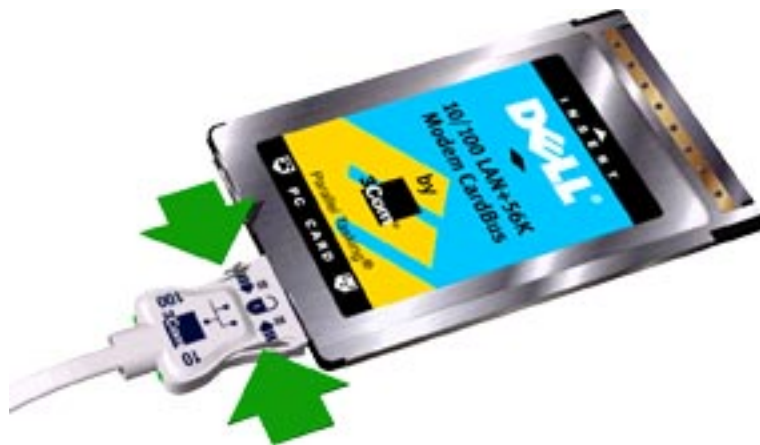
Figure 6 Disconnecting Cables from the Card
