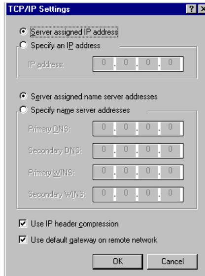
If your ISP provided you with an IP address for your computer, select **Specify an IP address** and enter the static address in the box provided. If your ISP requires you to enter an IP address for their name server (DNS), select **Specify name server addresses** and enter the IP addresses given to you by your ISP. Click **OK** to save the TCP/IP values and return to the **Server Types** tab.
