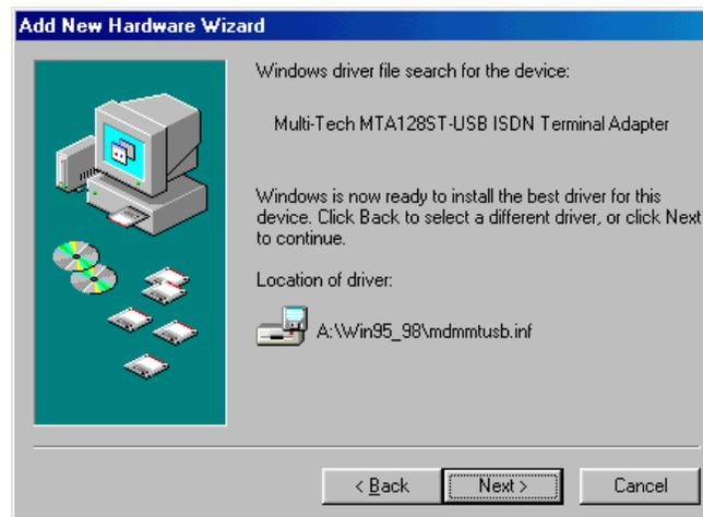
Windows selects the proper driver from the installation disk and displays the information for verification. Click **Next >** to install the selected driver.
