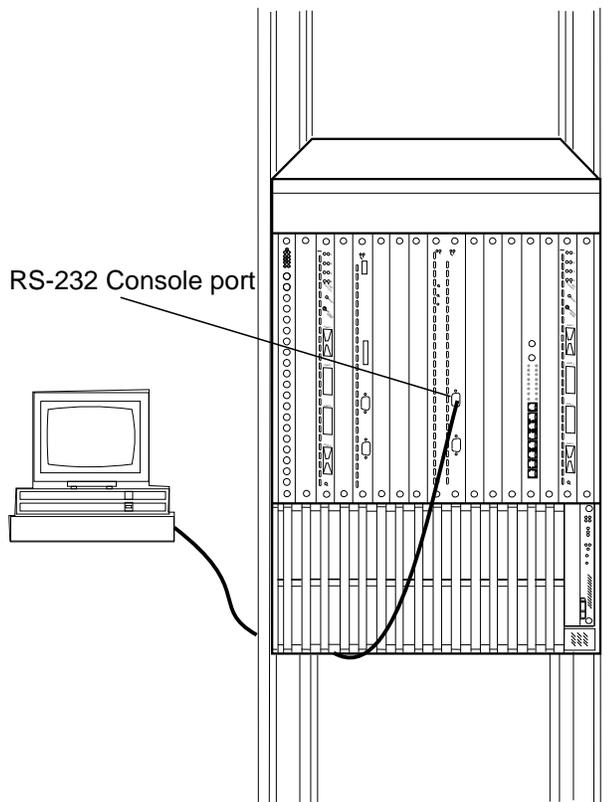
**Figure 2-3. Attaching a Terminal to the 6416SW RS-232 Console Port**
