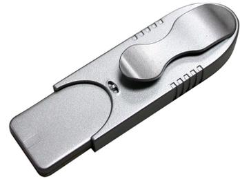
The X-Disk is a removable flash disk drive with USB connection and can support up to 512MB disk space, which is 355 pieces of 1.44MB floppy disk. The X-Disk is USB 2.0 compliant and is a plug-and-play device, you just simply plug it into any USB port and it will be automatically detected by the operating system as a removable drive. Now you can read, write, copy, delete and move data from your hard disk drive to the X-Disk and vice versa.
