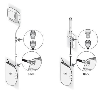
1 Position the antenna so that there are minimal obstacles between it and any client with which it will communicate. While maintaining a direct line of sight between the antenna and a client is not strictly necessary, such an arrangement helps to
