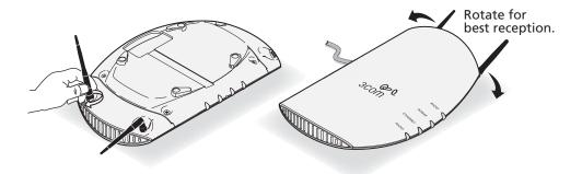
Depending on the coverage required for your site, you may want to replace the standard detachable antennas with one of the external antennas available for use with the access point. See "Selecting and Connecting a Different Antenna Model" on page 22.
