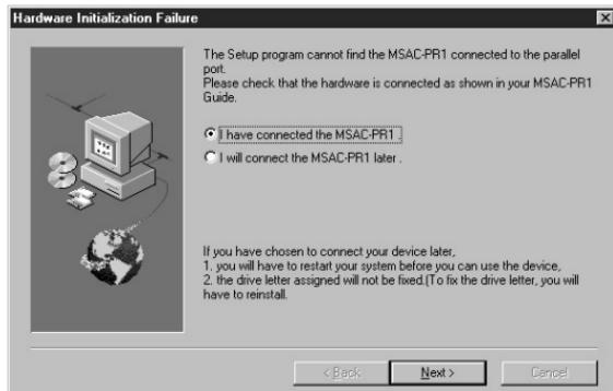
If the “Removable Disk” icon does not appear on restarting the PC even with the PC card inserted, it may be that the BIOS settings in the PC are not set correctly for MSAC-PR1. You will need to change the BIOS settings.
