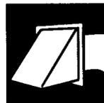
Is exhaust vent or outside exhaust hood clogged with lint? Refer to venting section on pages 6-7.
