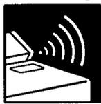
The lint signal (a whistle tone) indicates excessive lint is present on your lint screen, or it has a residue buildup. See page 19. A full lint screen restricts airflow and reduces drying efficiency. When you hear the signal, stop the dryer and clean the lint screen.
