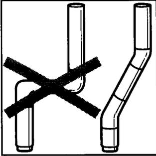
5. Use duct tape to seal all joints. **Do not** use screws to secure vent. Lint may catch on screws.
