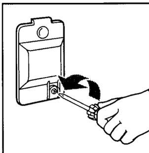
from the back wall of the dryer by removing the screw located in the lower right corner of the cover.
