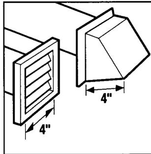
3. The exhaust vent can be routed up, down, left, right, or straight out the back of the dryer. Space requirements are listed in your Installation Instructions.
