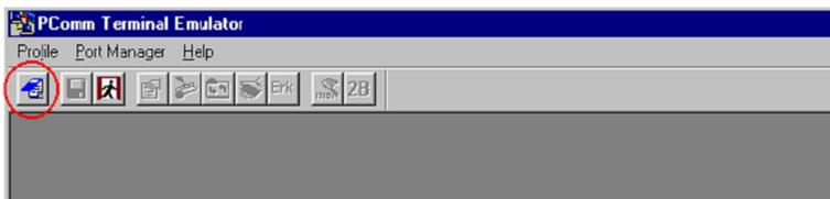
4. The **Property** window opens automatically. From the **Communication Parameter** page, select the appropriate COM port for the connection, **COM1** in this example, and **38400** for **Baud Rate**, **8** for **Data Bits**, **None** for **Parity**, and **1** for **Stop Bits**.
