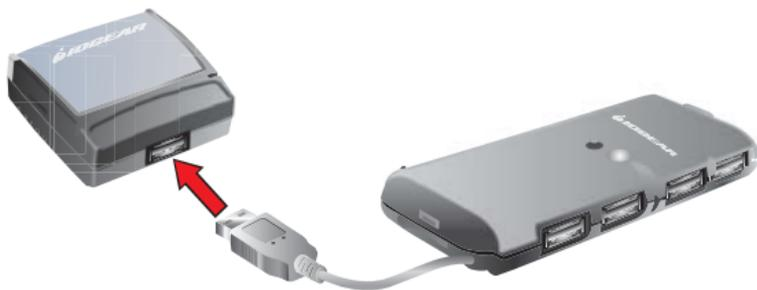
Note: USB Net ShareStation can only support up to 4 USB devices through a USB 2.0 Hub and certain USB devices require a direct connection to your computer in order to function at full capacity.
