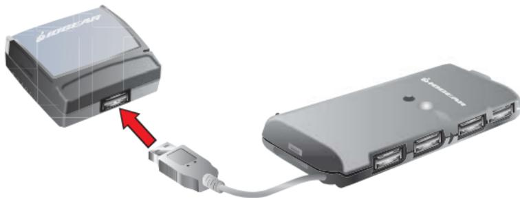
Please note that the USB Net ShareStation can only support up to 4 USB devices through a USB 2.0 Hub and certain USB devices require a direct connection to your computer in order to function at full capacity.
