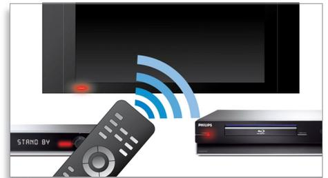
EasyLink lets you control multiple devices like DVD players, Blu-ray players, TV's etc. with one remote. It uses HDMI CEC industry-standard protocol to share functionality between devices through the HDMI cable. With one touch of a button, you can operate all your connected HDMI CEC enabled equipment simultaneously. Functions like standby and play can now be carried out with absolute ease.
