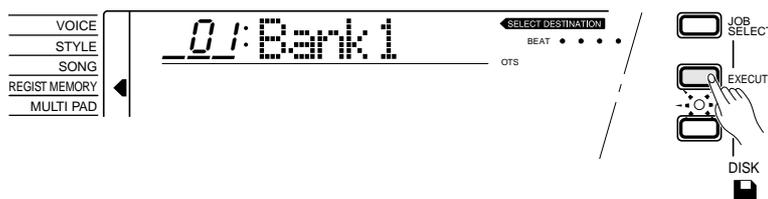
"Loading" will appear on the display while the data is being loaded. When the data has been loaded the [EXECUTE] indicator will go out.
