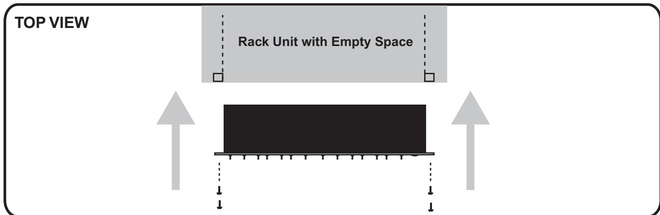
The CLG-600 mounts in a standard 19-inch equipment rack. The mounting screw threads vary with different rack manufacturers and you should refer to your rack instructions for proper hardware. An oval head or flat head screw with a plastic countersink washer is preferred to protect the finish of the CLG-600 under the screw. The CLG-600 is housed in a rugged steel case and can tolerate "in the field" abuse, however proper care will best suit the unit for long-life and performance.
