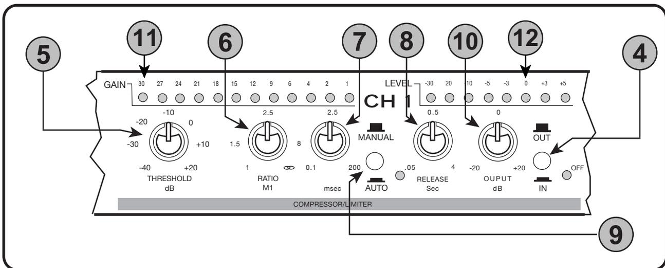
**6. RATIO control** - This control determines the RATIO of change in **output level** to changes in **input level** for all signals above threshold. The numbers printed around the RATIO control are calibrated in dB and indicate the increase in input (above threshold) required to produce a 1db increase in output. This can be expressed conveniently as a ratio. If the **output** remains constant no matter how high the input level, we have an infinite input/output ratio.
