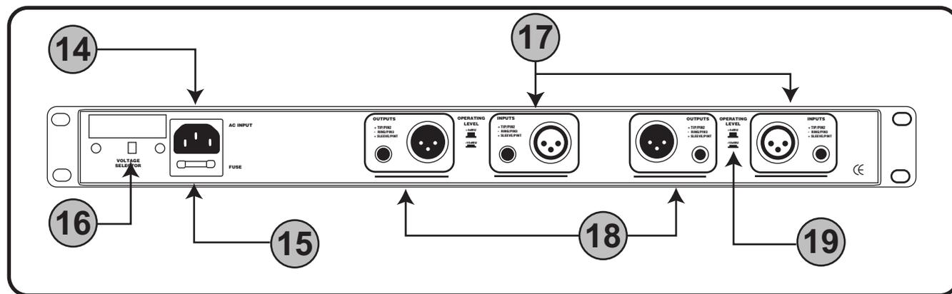
**14. AC POWER terminal** - This terminal is where the MAINS POWER CABLE is connected.
