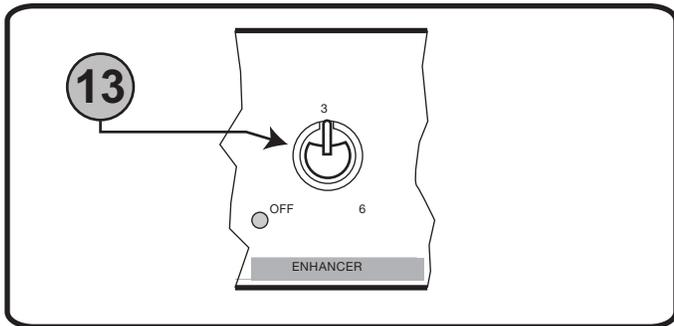
**13. PROCESS control** - This control sets the available amount of ENHANCEMENT between OFF and 6. DYNAMIC ENHANCEMENT allows you to replenish any high frequencies that may have become lost during the compression process. ENHANCEMENT should only be added when compression is taking place.
