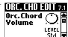
This is a relative parameter, which means that its value is added to or subtracted from the standard value ("Std").
