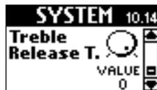
term "Release" is taken from synthesizers and refers to the speed at which the notes you play disappear when you release the keys.
