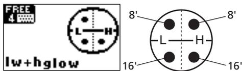
"L" refers to the low range and "H" to the high range. The exact ranges depend on the FREE BASS mode you selected. See also the illustration on page 71 where the high range is indicated by means of black buttons, and the low range by means of white buttons.
