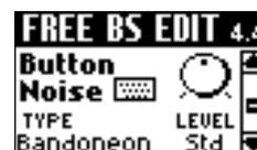
can select the instrument whose button noises should be used when you select this register. (Note that other Free Bass registers can be assigned different noises.)
