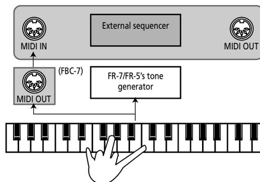
If the FR-7/FR-5 is used as tone generator for an external sequencer, you must connect the sequencer's MIDI OUT socket to the FBC-7's MIDI IN port (because MIDI data always go from OUT to IN).
