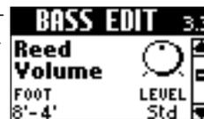
This is a relative parameter, which means that its value is added to or subtracted from the standard value ("Std"). As a rule, it would be wise to decide which reed is most important and set its Volume parameter to "Std". Then reduce or increase the volume of the "ancillary" reeds to create the desired balance.
