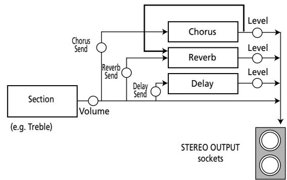
■ **Chr►Dly (0~127)**—This parameter sets the amount of chorus sound that is sent to the Delay processor. Higher values result in more sound being sent. The value "127" effectively allows you to connect the Chorus and Delay effects in series (Chorus before Delay). If you do not want the chorus signal to be processed by the Delay effect, set this value to "0".
