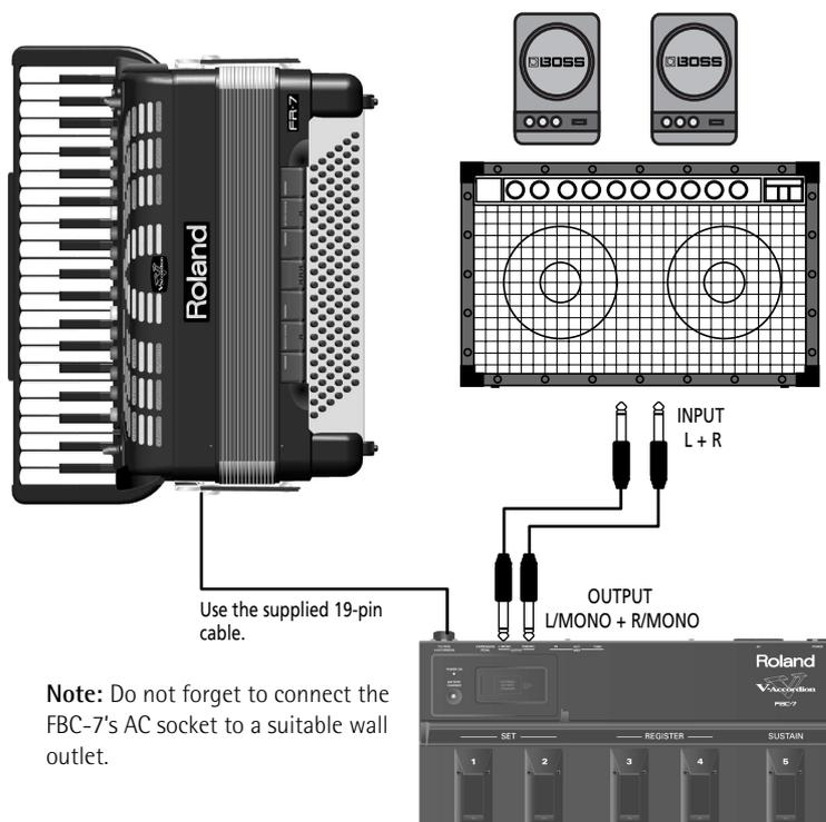
**Note:** Do not forget to connect the FBC-7's AC socket to a suitable wall outlet.
