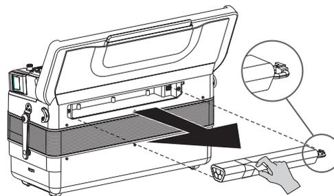
The battery is connected to the FR-7/FR-5 by means of a cable. You need to disconnect the cable from the battery by pressing the clip on the connector before fully removing the battery.
