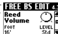
This is a relative parameter, which means that its value is added to, or subtracted from the standard value ("Std"). As a rule, it would be wise to decide which reed is most important and set its Volume parameter to "Std". Then reduce or increase the volume of the "ancillary" reed to create the desired balance.
