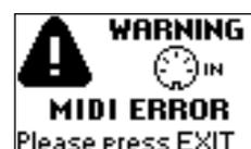
Press **[EXIT/JUMP]** to return to the Main page, reduce the speed at which the data are transmitted by your sequencer, and try again. If that does not help, check the data file you are transmitting.
