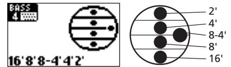
These indications refer to the octaves (vertical direction) and the number of slightly detuned reeds that are used (horizontal direction).
