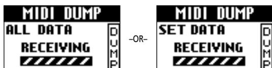
**Note:** When transmitting an "ALL DATA" file to the FR-7/FR-5, wait until the "WRITE COMPLETE" message appears before stopping playback on your sequencer. Failure to do so will render your FR-7/FR-5 inoperable. If that happens, you need to initialize it (see "Restoring the factory defaults" on p. 94).
