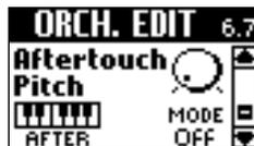
that you press a key even further down after playing a note. This effect allows you to bend the pitch down (temporarily lower the note) by a quarter ("1/4 Down") or a semi-tone ("1/2 Down"). Select "1/4 Up" or "1/2 Up" to bend the notes up a quarter or a semi-tone. Select "Off" to switch off the Orchestra section's aftertouch recognition.
