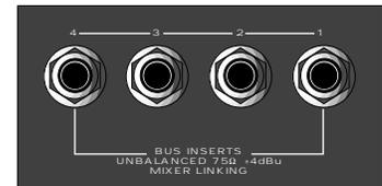
All MPL 1204 insert jacks accept 1/4" TRS plugs, with the ring carrying the send signal and the tip carrying the return signal; this will normally be connected to a Y-cord (see the “Connecting The MPL 1204” section on page 12 in this manual for a wiring diagram). This configuration is sometimes known as an “effects loop,” since the signal is sent and returned over the same cable.
