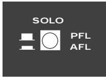
The MPL 1204 provides two options for soloing input signals in headphones connected to the front panel headphone jack—*Pre Fade Listen (PFL)* and *After-Fade Listen (AFL)*. The Solo switch in the main section (#8 on page 7) allows you to choose between these two modes of operation. Although they may at first glance appear similar (and although both are non-mix-destructive), there is in fact a significant difference between the two.
