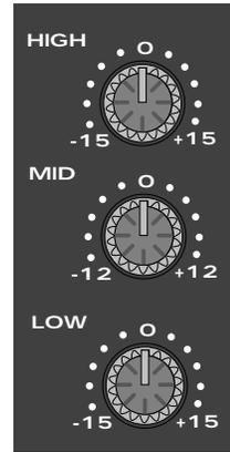
When an EQ knob is in its center detented position (“0”), it is having no effect. When it is moved right of center, the selected frequency area is being boosted; when it is moved left of center, the frequency area is being attenuated.
