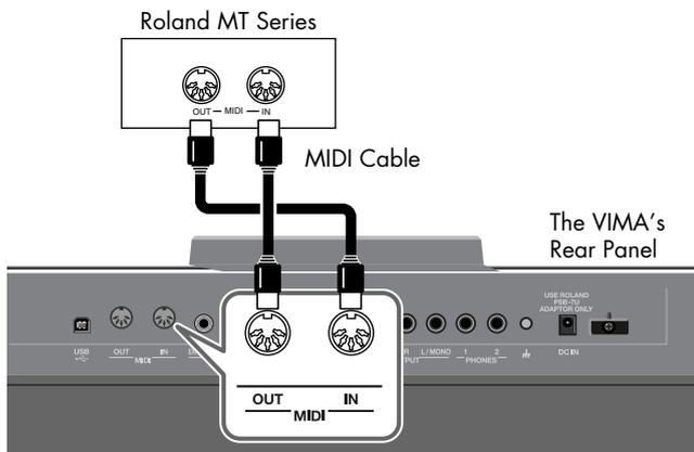
**NOTE** If you connect the VIMA with a MIDI sequencer, turn off the Thru function of the connected MIDI sequencer.
