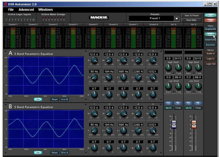
If two bands are set to the same frequency, the gain settings are additive and the response curve may go off the display. The response is not limited to the display scale, and the 32-bit floating-point processors accurately calculate the combined response of all five bands.
