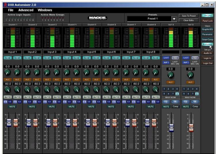
One of the dangers of using a conventional mixer in a sound system operated by an untrained sound technician is the occurrence of feedback. The more open channels there are, the greater the overall system gain and the lower the potential acoustic gain (gain before feedback).
