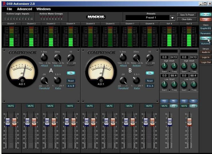
Click this button to open the Compressor window for the A and B outputs. Each compressor has five knobs: Attack, Release, Threshold, Ratio, and Output. Click and drag on the individual knobs to adjust each parameter. An analog-style meter indicates the amount of compression applied in decibels.
