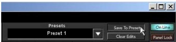
The "Save To Preset" window opens. Enter a name for each preset in this window, then click on the Save To Preset button to save it.
