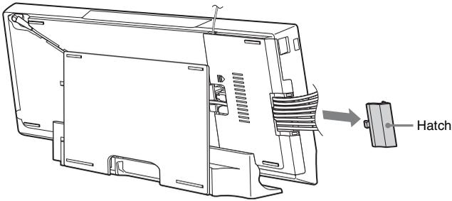
To open the hatch, remove the panel cover, hold the hatch, and then pull it up and outward.
