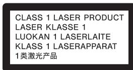
This appliance is classified as a CLASS 1 LASER product. This marking is located on the rear exterior.
