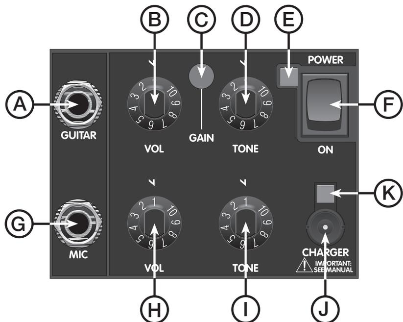
**A. GUITAR INPUT** - Plug your guitar in here. This is a 1/4 inch, high impedance input for electric guitars.
