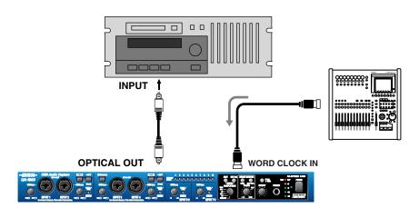
\* If the word clock input connector and the digital input connector are both connected, the word clock input connector will take priority for synchronization.
