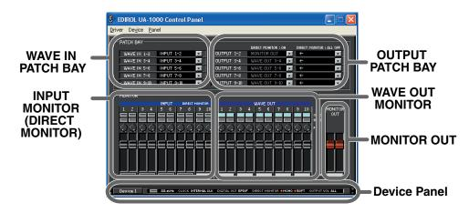
You can use UA-1000 Control Panel to control each block of the UA-1000.
