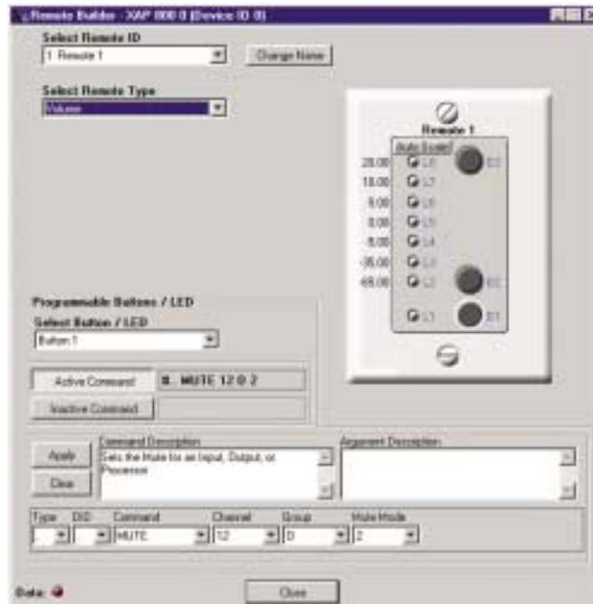
Figure 6.5. Volume Panel selected in the Remote Builder
