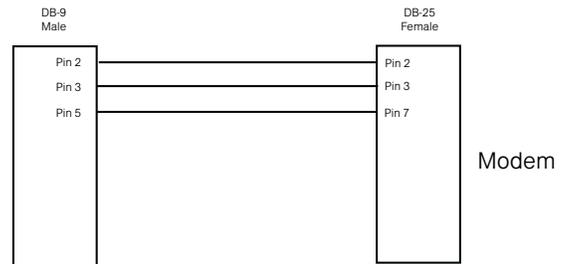
Figure B.3. XAP 800 to Modem RS-232 Connections
