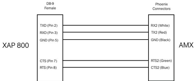
Figure B.4. XAP 800 to AMX RS-232 Connections
