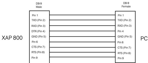
Figure B.2. XAP 800 to PC RS-232 connections
