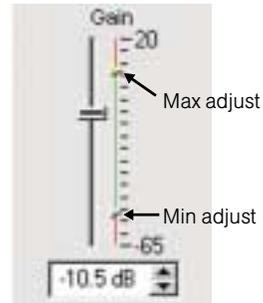
Figure 3.46. Gain adjust on line level input
