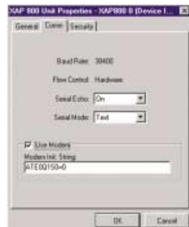
Figure 3.13. Unit Properties Comm tab
