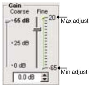
Figure 3.42. Gain adjustment
