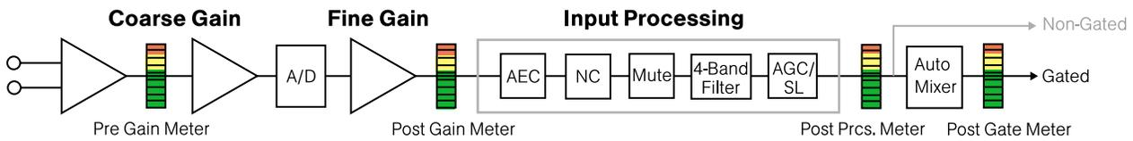
Figure 3.43 Meter locations in the Inputs 1-8 signal path
