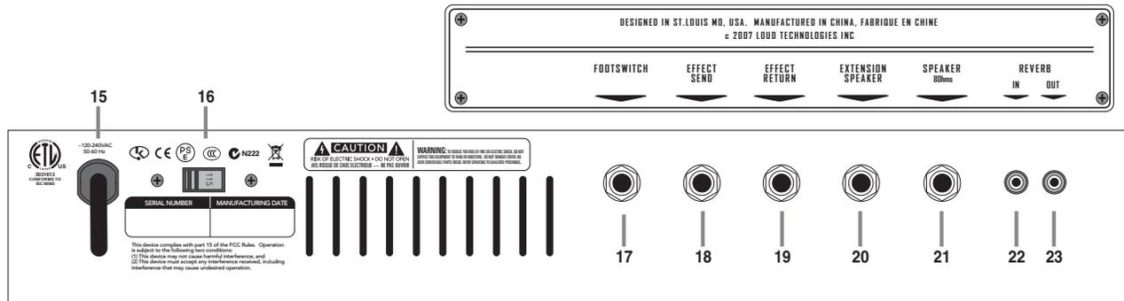
**15. AC LINE CORD:** The grounded power cord should only be plugged into a grounded power outlet that meets all applicable electrical codes, and is compatible with the voltage, power, and frequency requirements stated on the V50-112 rear panel. Do not attempt to defeat the safety ground connection.
