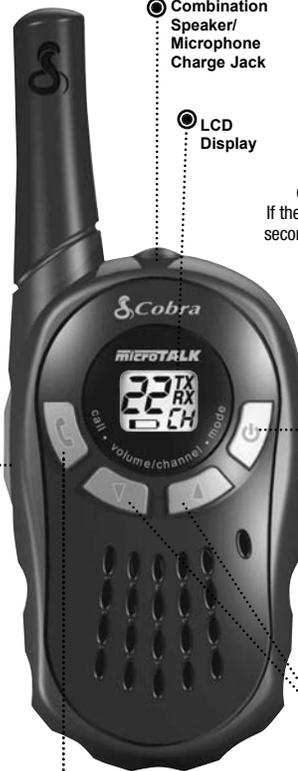
While in **Standby** mode or when selecting a channel, shows current channel (1 through 22).
