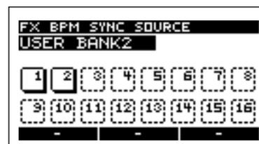
3. Press the pad to specify the sample that is to be the sync source.
