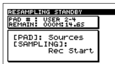
**5. As necessary, switch the pad bank (p. 30), and press the pad(s) for the sample(s) that you want to resample (the Source Pads).**
