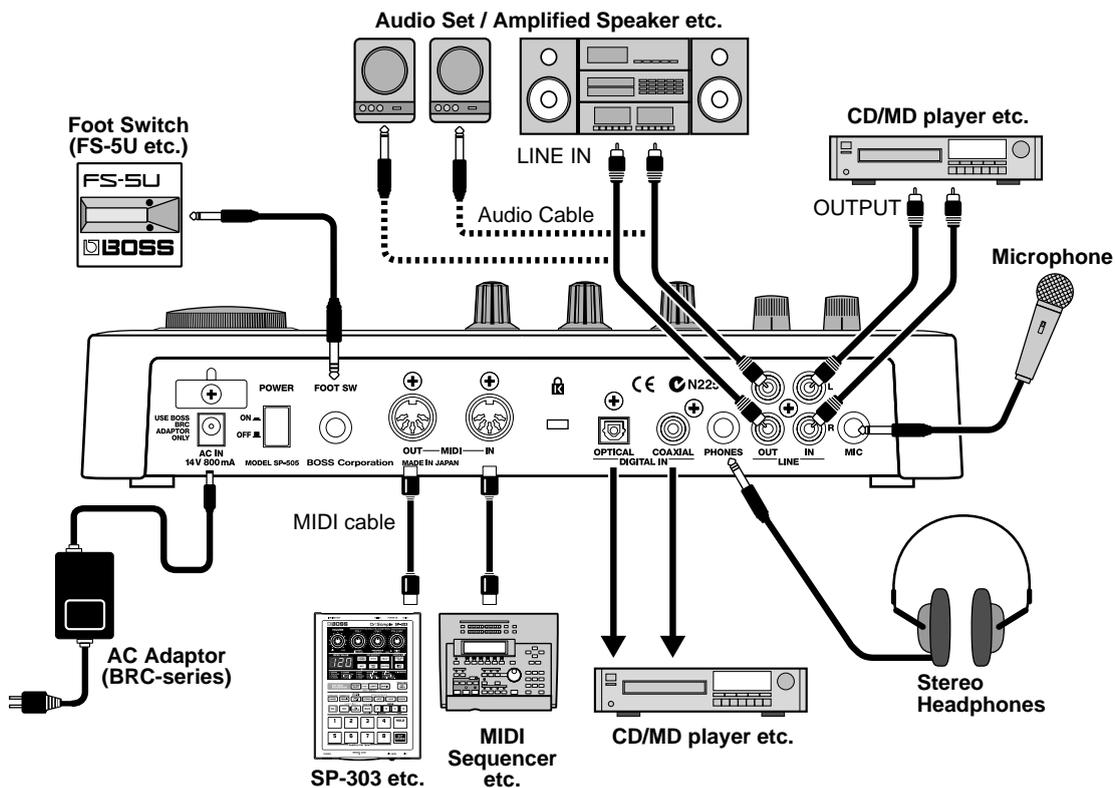
\* To prevent malfunction and/or damage to speakers or other devices, always turn down the volume, and turn off the power on all devices before making any connections.
