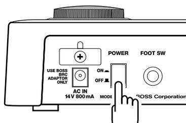
This unit is equipped with a protection circuit. A brief interval (a few seconds) after power up is required before the unit will operate normally.
