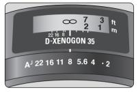
Setting the aperture to "A"(Auto) Turn the aperture ring to align the aperture-A index with the line while depressing the Aperture-A-lock button. The aperture ring can be released from "A" in the same manner to set your desired f-stop manually.
