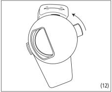
**Note:** Unless the locking tab on the continuous flow attachment is engaged, the unit will not turn on.
