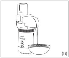
9. Rest the food pusher in the feed tube. Now, holding the food pusher with one hand and the feed tube with the other, turn the continuous flow attachment to the left (anti-clockwise) until the large tab slides into the horizontal slot at the back of the processor body. This will engage the automatic switch and the food processor will turn on (12).
