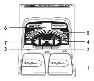
I. Footswitches - These 2 Footswitches are used to select presets, access the Tuner, or bypass the RP50. The Up Footswitch increments, and the Down Footswitch decrements through the presets. Pressing both Footswitches simultaneously bypasses the selected preset. Pressing and holding both Footswitches accesses the Tuner.
