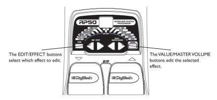
When the stored value of an effect is changed, the lower right decimal point in the display lights indicating you need to store the changes. Changing presets, or turning the power off before storing any changes will erase any changes made and revert to the stored values for the preset.
