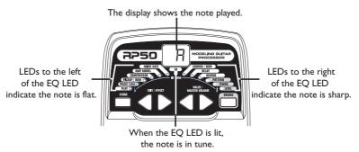
When the Tuner is enabled, you can change your tuning reference. The default factory setting is A=440 Hz. (displayed as 40). Press the Value Buttons to select alternate dropped tunings. Alternate tunings are A = Ab (displayed as  $\Pi$ b), A = G (displayed as  $\Pi$ ), and A = Gb
