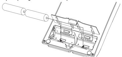
Connecting a cable to the Input applies power to the RP50. Disconnecting your instrument from the Input of the RP50 disconnects the battery power. Turn your amplifier(s) on and adjust the volume(s) to a normal playing level. To prolong the battery life, disconnect your instrument from the RP50's Input when not in use .
