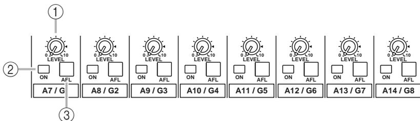
These output channels control the signals of AUX buses 7–14 or GROUP buses 1–8. You can use the GROUP/AUX FLIP switch (page 14) to select the signals that will be controlled.
