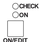
In Check mode, pressing an ON/EDIT switch will switch the lit/dark status of the CHECK indicator. The actual on/off setting (the setting of the ON indicator) will not be affected.
