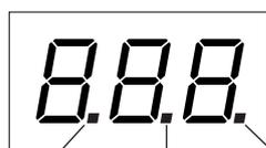
This will light if the display shows a scene memory number in which no scene has been stored. If not even one scene has been stored in scene memory, this dot will light when the power is turned on.
