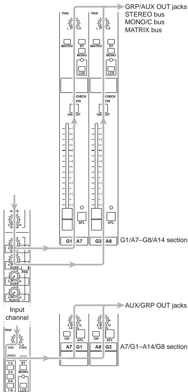
When you change the setting of the GROUP/AUX FLIP switch, numerous functions of the output channels of GROUP buses 1–8 and AUX buses 7–14 will change in addition to the faders. The functions available for the output channels of each bus are shown below for each setting (GROUP/AUX) of the GROUP/AUX FLIP switch.
