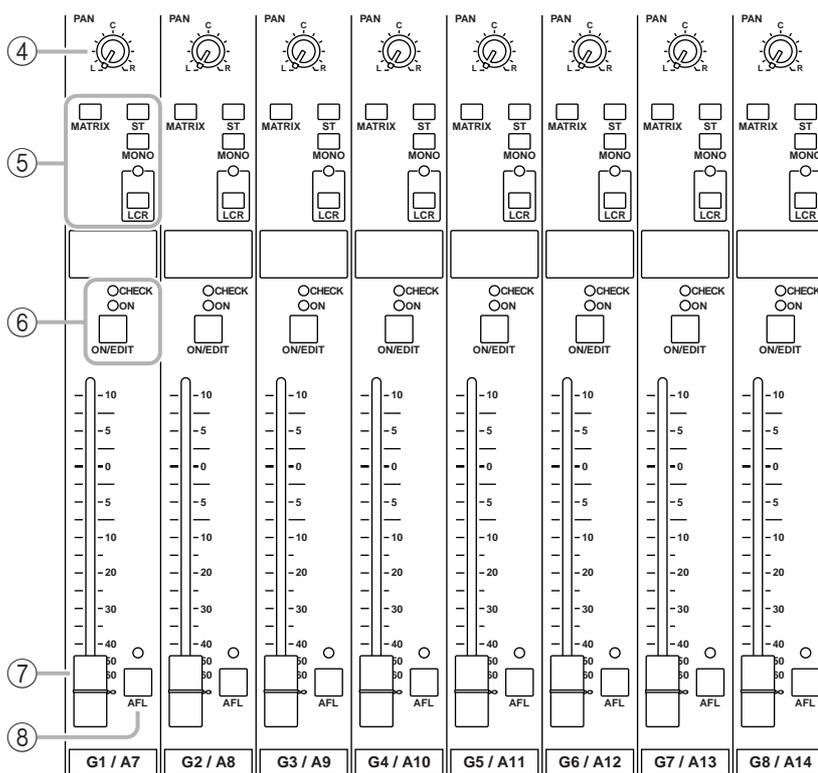
These are the output channels that control GROUP buses 1–8 or AUX buses 7–14. Use the GROUP/AUX FLIP switch (page 14) to select which signals will be controlled.
