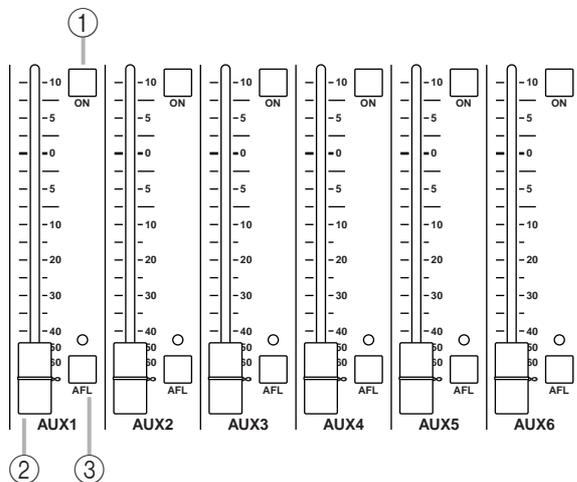
These are the output channels that control the signals of AUX buses 1–6. The signals that have passed through these output channels will be output individually from the AUX OUT 1–6 jacks (page 27). In addition, they pass through the MONITOR MASTER PFL/AFL buses and can be monitored from the MONITOR OUT L/R and the PHONES jacks.
