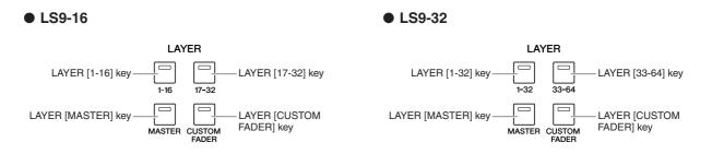
In conjunction with this difference, there are also differences in the numbering of the channel modules on the panel and the channels that are assigned to each fader layer.
