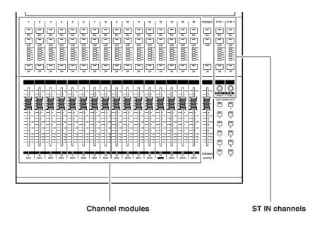
The LS9-16 provides thirty-two channel modules and four ST IN channels. By switching fader layers you can operate up to sixty-four INPUT channels (monaural).
