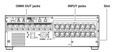
In contrast, the rear panel of the LS9-32 provides thirty-two INPUT jacks, sixteen OMNI OUT jacks, two slots, and one LAMP connector.
