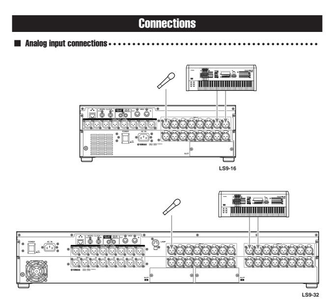
Connect microphones or line level devices to INPUT jacks  $1-16 \{1-32\}$ . When the LS9 is in its initial state, the signal from each INPUT jack is patched to the following channels.
