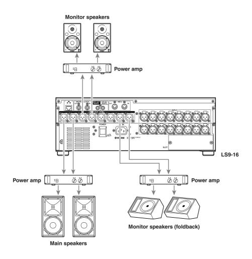
OMNI OUT jacks 1-8 {1-16} can be connected to your main speakers, monitor speakers (foldback), or monitor speakers for the engineer.
