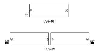
Separately sold mini-YGDAI I/O cards can be installed in these slots to provide additional input/output ports. The LS9-16 has one slot, and the LS9-32 has two slots. Each slot can input/output a maximum of 16 channels of signals.
