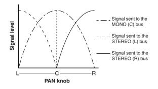
If a ST IN channel is selected, operating the TO ST BALANCE knob will change the signal levels sent from the ST IN L/R channels to the STEREO (L/R) bus and MONO (C) bus as shown in the following illustration.
