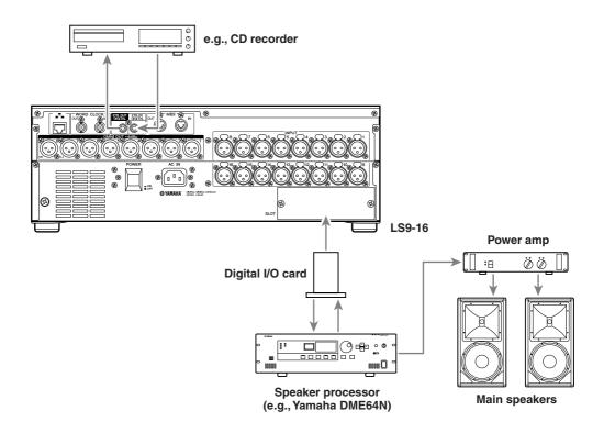
Use the 2TR IN DIGITAL/2TR OUT DIGITAL jacks or the mini-YGDAI slot to send or receive digital audio signals between the LS9 and external equipment. When the LS9 is in the default state, the signals of the following channels are patched to the 2TR IN DIGITAL/2TR OUT DIGITAL jacks and slots. This patching can be changed as necessary ( $\rightarrow$  p. 95, 99).
