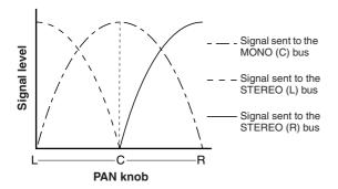
If a stereo MIX channel is selected, operating the TO ST BALANCE knob will change the signal levels sent from the MIX channel to the STEREO (L/R) bus and MONO (C) bus as shown in the following illustration.
