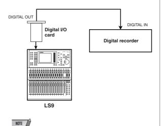
If you install a digital I/O card in a slot and digitally connect an external device, you must synchronize the word clock of the LS9 and the external device (→ p. 46).
