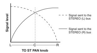
If a ST IN channel is selected, operating the TO ST BALANCE knob will change the signal levels sent from the ST IN L/R channels to the STEREO (L/R) bus and MONO (C) bus as shown in the following illustration. In this case, the [PAN] encoder will operate as a conventional BALANCE knob, and no signal is sent to the MONO (C) bus.
