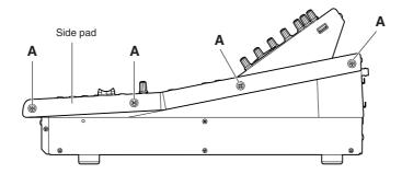
3 At the locations indicated by the arrows, tighten the screws to attach the rackmount hardware.
