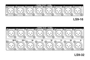
These are XLR-3-32 male output jacks for outputting analog audio signals. These are used mainly to output MIX/ MATRIX channel signals. The nominal output level is +4 dBu.
