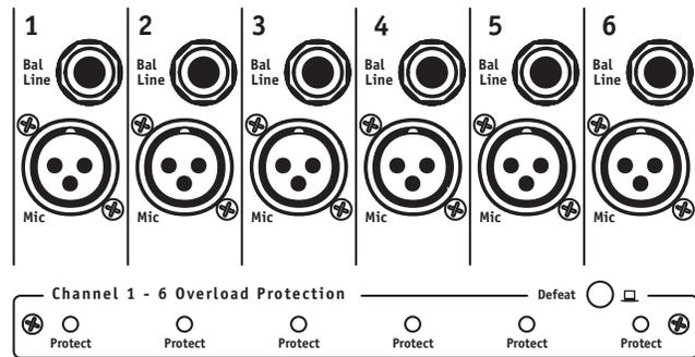
Each channel features a Protect LED to indicate when the overload protection is working. A single Defeat switch activates this feature on a group of six channels simultaneously.
