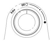
Your blender offers a 2 speed range controlled by the rotary knob. The blender will operate until you rotate the dial to Off / **O**. Turn the dial to Pulse for instant control of blending.
