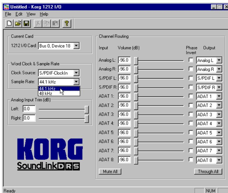
This should be set to the same sample rate as the 328XD was set to in the 'Wordclock' section in chapter 2 of this manual. If the 328XD and 1212 are set to different sample rate settings, audio from the 1212 will play back at the incorrect speed.
