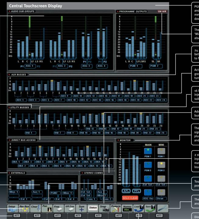
PGM outputs provide 2 outputs in stereo and/or 5.1, with dynamics gain reduction meters and simultaneous stereo and mono downmix feeds
