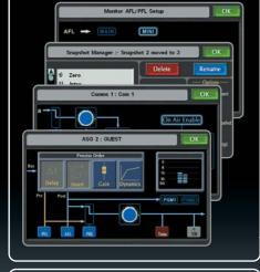
Reverse Bus feature allows overview and control of channel contribution to selected bus
