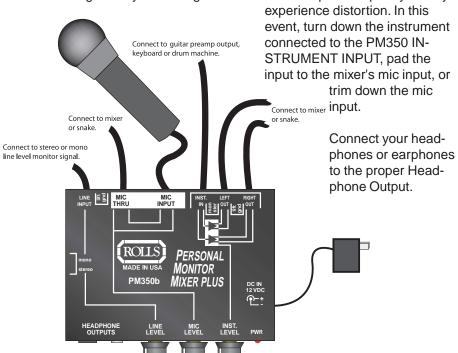
Make sure the Rolls PS27 12VDC power supply is connected to an active AC outlet, and all audio connections are in place.
