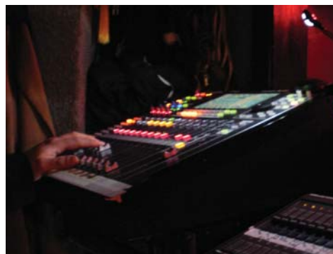
The RSS M-380 V-Mixer mixes live sound and provides audio for recording split.
