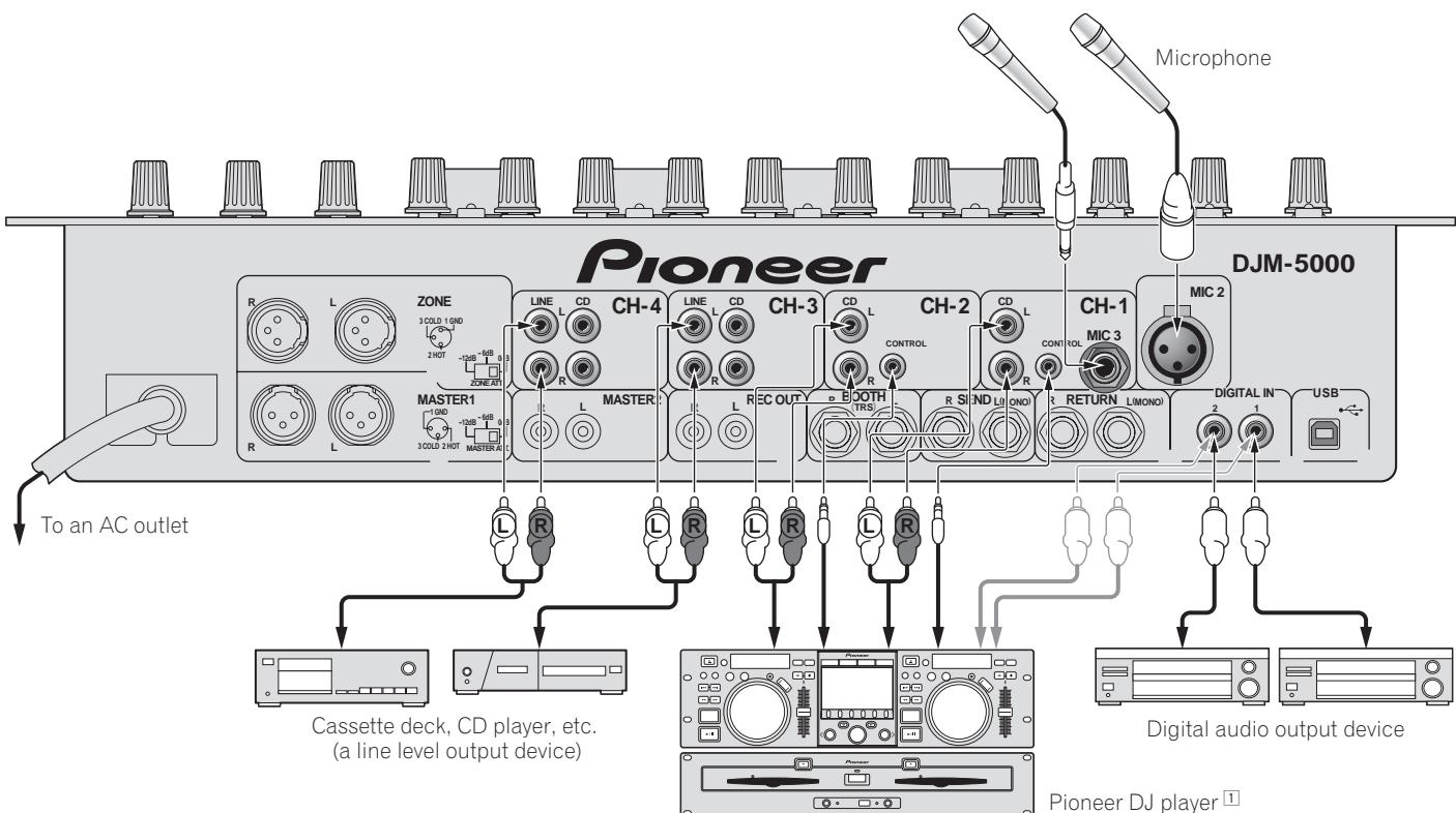
[1] Connect a control cable to use the fader start feature (page 14).
