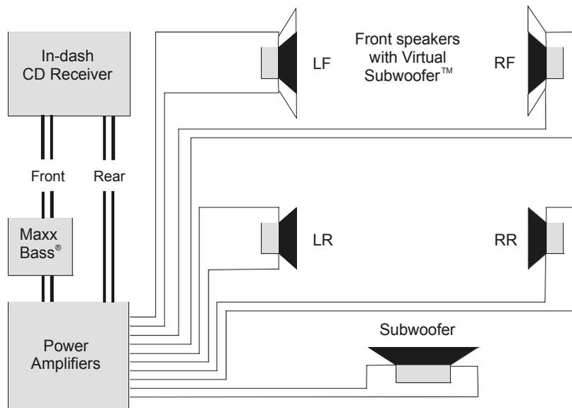
**WARNING:** If you are using a source unit with bridged high powered (or "floating ground") speaker outputs, a suitable high to low level adapter must be used. If you are unsure about your head unit see your local *PrecisionPower™* dealer.
