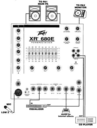
XR 680E external EQ & internal power amp for mains. Internal EQ & internal power amp for monitors.
