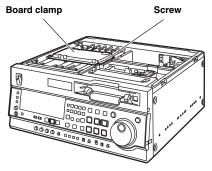
4 Insert the analog video input board into the slot marked F2 located on the rear panel side of the VTR.
