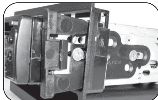
**NOTE:** When reinstalling the screws into the bottom of the 99-5806 use the (2) supplied Phillips screws instead of the factory screws removed in step 5 in Dash Disassembly.
